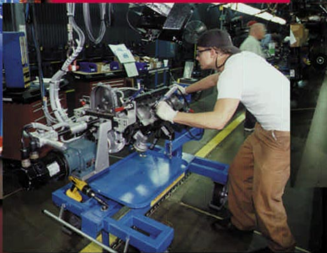
Computerized engine pressure check system
